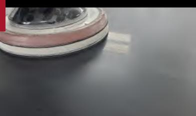
Further refine sand-scratches with 3000-grit foam pad and water on a 6" DA sander.
