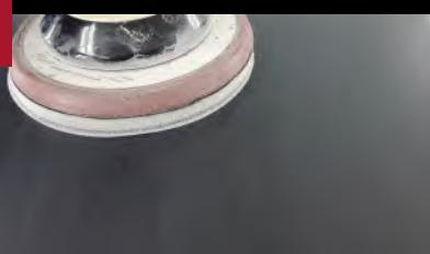
Remove paint defects using 1500-2000 grit sandpaper on a 6" DA sander.
