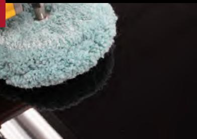
Compound the area using **Performance Cutting Compound** on a **Green Foam Pad**.
