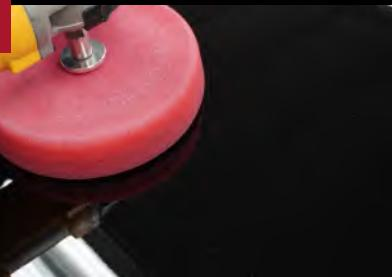
Polish the area using **Performance Finishing Polish** on a **Red Foam Finishing Pad**.
